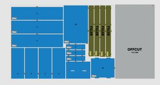
Cut in small pieces the remaining material to simplify manual offcut handling or automatic extraction.
