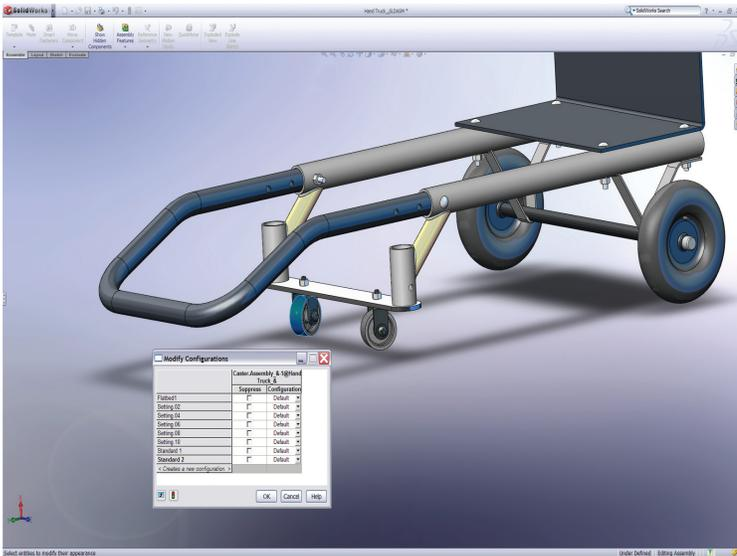
With SolidWorks software you can speed the creation of multiple configurations.
