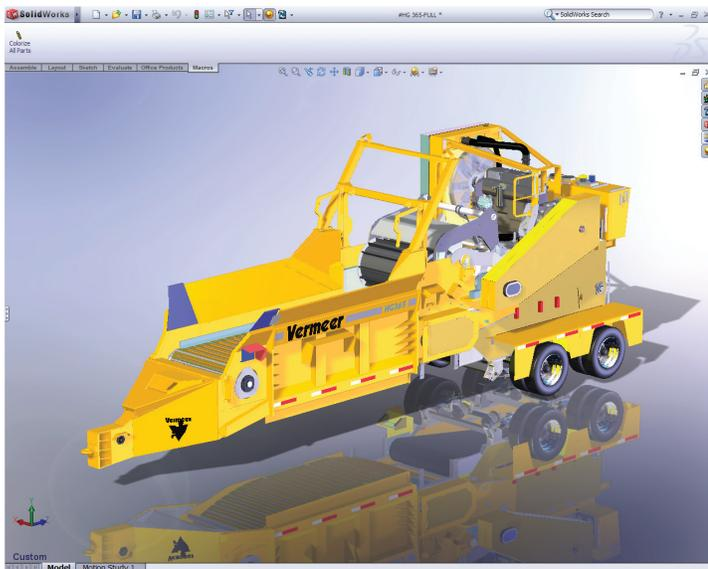
Vermeer uses SolidWorks software to check for interferences and collisions in large assembly designs, which range from 500 to 4,000 parts.
