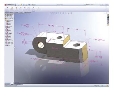
DimXpert provides automated dimensioning and tolerancing in 3D per industry standards. Dimensions and tolerances are created with the correct syntax and semantics, and graphical feedback is provided to let you know when your model is fully dimensioned and toleranced.
