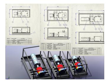
DriveWorksXpress automates repetitive design tasks by capturing valuable design rules inside SolidWorks software and automatically generating assemblies, drawings, and models.
