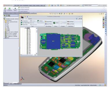
The CircuitWorks capability enables bidirectional collaboration between electrical and mechanical design engineers to ensure that printed circuit boards PCBs fit and function in mechanical products.
