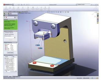
With TolAnalyst, you can verify tolerances and dimensioning schemes, and then quickly make necessary changes until you achieve the desired tolerance stack-up results.
