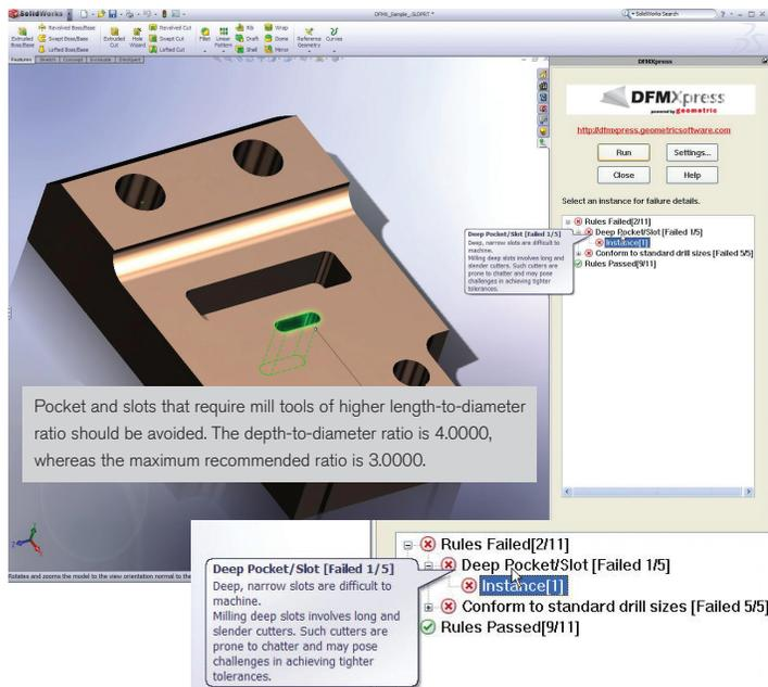
Using SolidWorks CAD software and DFMpress, you can fully interrogate the manufacturability of your designs to make sure that they are ready to be manufactured. Combined with other SolidWorks Simulation tools, the software can help you build a specialized Design for Manufacturability business.
