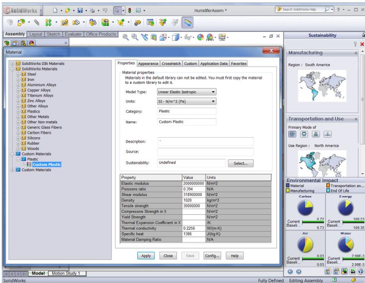
With SolidWorks Simulation tools, such as the SolidWorks Sustainability package shown here, you can extend your range of capabilities. SolidWorks Sustainability software lets you evaluate the environmental impacts that a design will have throughout its lifecycle.
