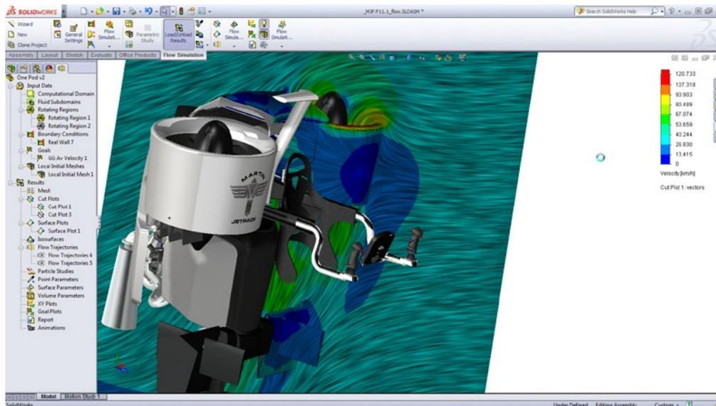
CAD embedded CFD Simulation
