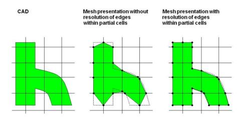
Figure 7: Mesh representation of CAD geometry with resolution of solid edges within partial cells.
