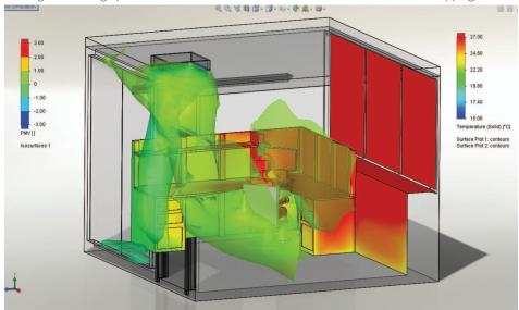
With the SolidWorks Flow Simulation HVAC Module, designers can fully assess the thermal environment created in an occupied zone by heating and cooling systems, including the calculation of comfort parameters.
