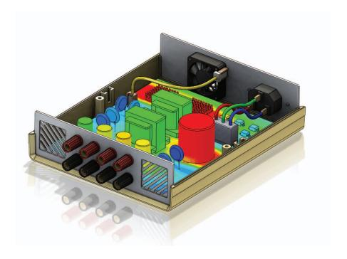
The SolidWorks Flow Simulation Electronics Cooling Module enables designers to evaluate the thermal properties of components and more accurately establish cooling requirements for PCB and enclosure designs.
