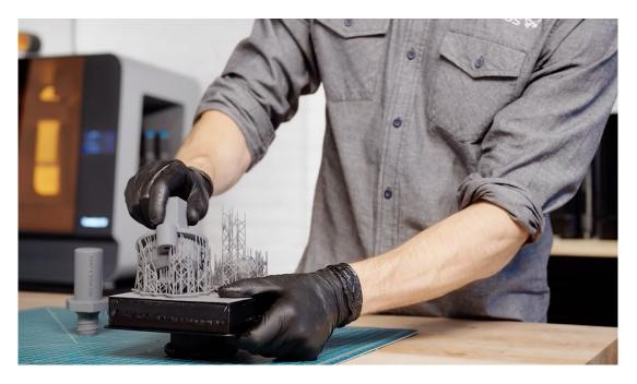
After the print is finished, there are three main steps in post-processing stereolithography parts: rinsing in isopropyl alcohol (IPA), removal of supports, and post-curing. Formlabs has made each of these steps as easy as possible to save you time and increase your throughput.
