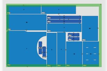
Our nesting solution also offers strategies such as minimizing the cutting force with the onion skin strategy and using the staydown contour operation, which optimize trajectories and save up to 20% of milling time.
